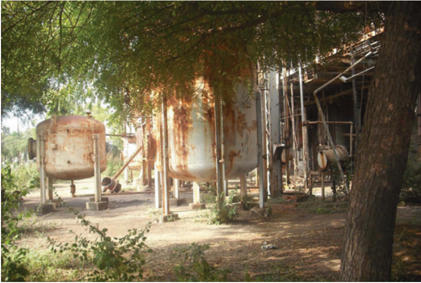
FIGURE 2. Degraded components of the Union Carbide pesticide plant in Bhopal, India. The site is now abandoned, but remains contaminated with pesticides, chlorinated benzenes, and heavy metals. Groundwater serving local communities is also contaminated.
