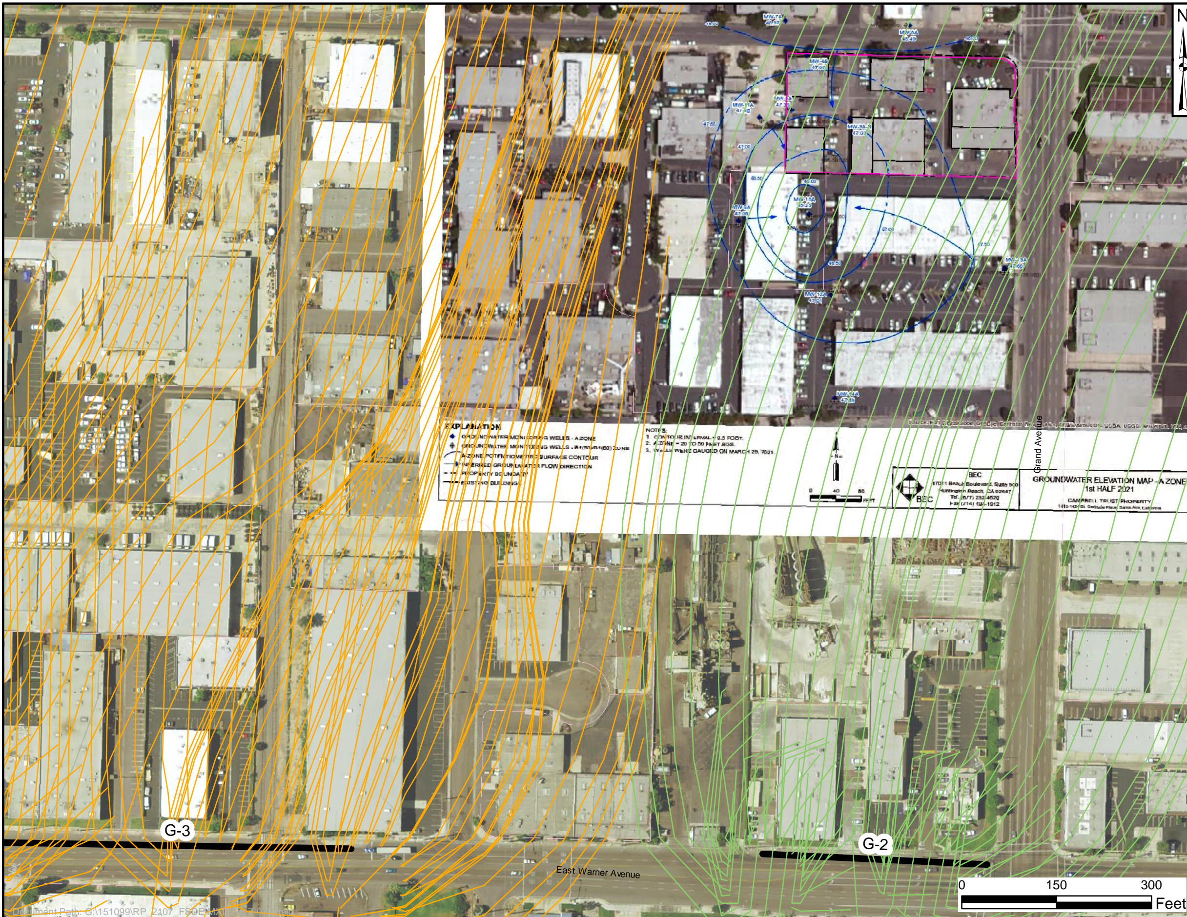
FIGURE 7-7A COMPARISON OF OCWD MODEL SIMULATED GROUNDWATER PARTICLE TRACKS VERSUS PUBLISHED A-ZONE GROUNDWATER ELEVATION CONTOURS, ALLAN T. CAMPBELL TRUST SOURCE SITE ORANGE COUNTY WATER DISTRICT SOUTH BASIN
