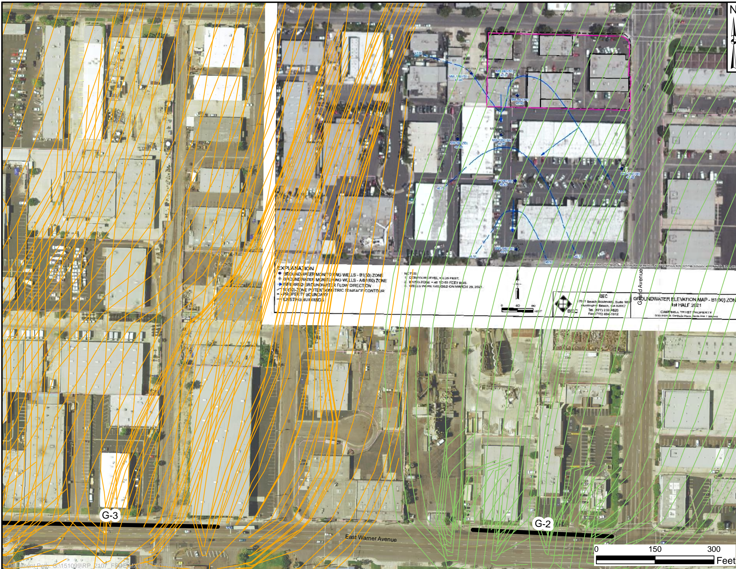
FIGURE 7-7B COMPARISON OF OCWD MODEL SIMULATED GROUNDWATER PARTICLE TRACKS VERSUS PUBLISHED B1(50)-ZONE GROUNDWATER ELEVATION CONTOURS, ALLAN T. CAMPBELL TRUST SOURCE SITE ORANGE COUNTY WATER DISTRICT SOUTH BASIN
