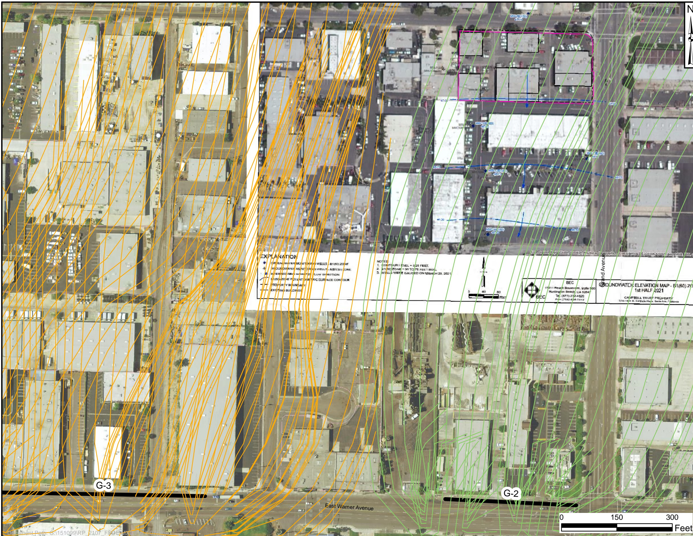
FIGURE 7-7C COMPARISON OF OCWD MODEL SIMULATED GROUNDWATER PARTICLE TRACKS VERSUS PUBLISHED B1(60)-ZONE GROUNDWATER ELEVATION CONTOURS, ALLAN T. CAMPBELL TRUST SOURCE SITE ORANGE COUNTY WATER DISTRICT SOUTH BASIN
